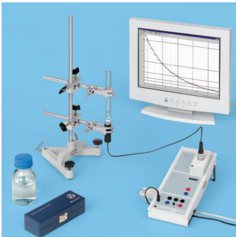
Determining the half-life of Ba-137m – recording and evaluating the decay curve using CASSY (P 6.4.3.4)
