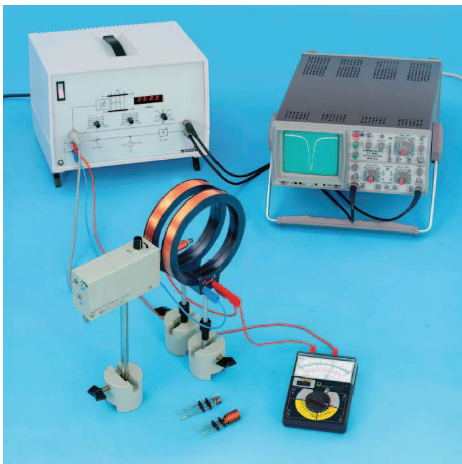
Electron spin resonance in DPPH – determining the magnetic field as a function of the resonance frequency (P 6.2.6.2)
