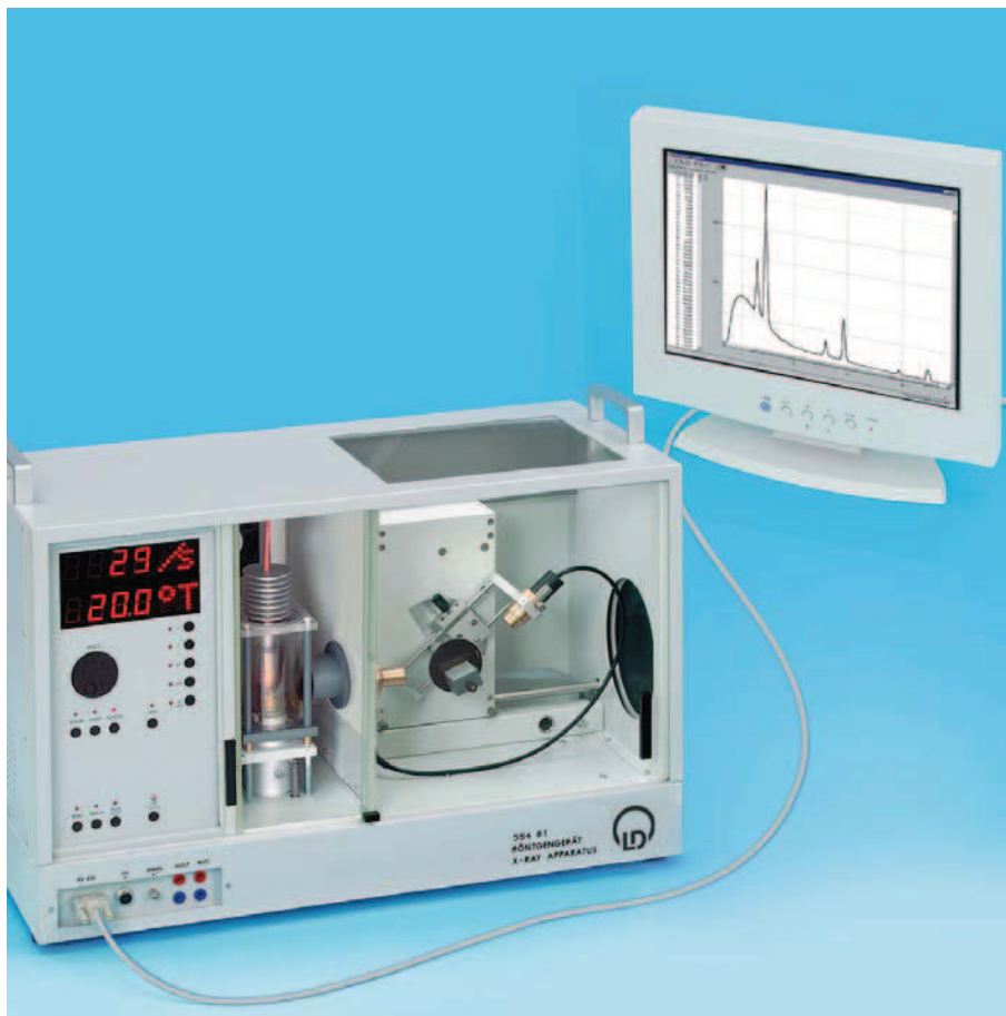
Bragg reflection: diffraction of x-rays at a monocrystal (P 6.3.3.1)
