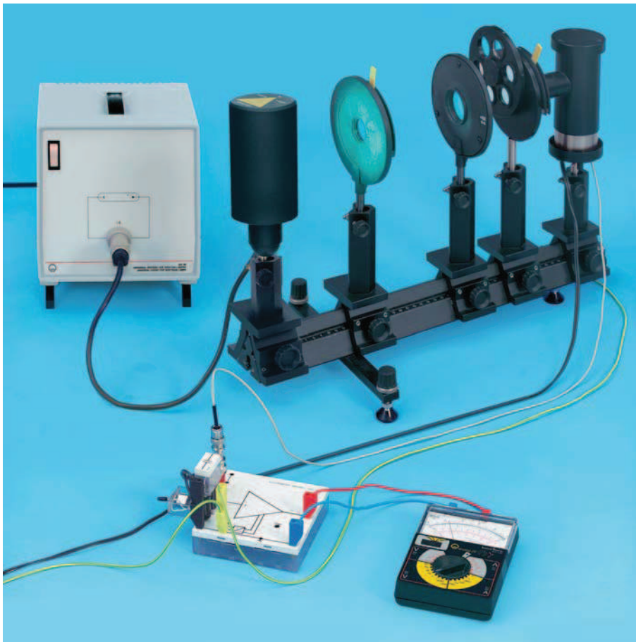
Determining Planck's constant – selection of wavelengths with interference filters on the optical bench (P 6.1.4.3a)
