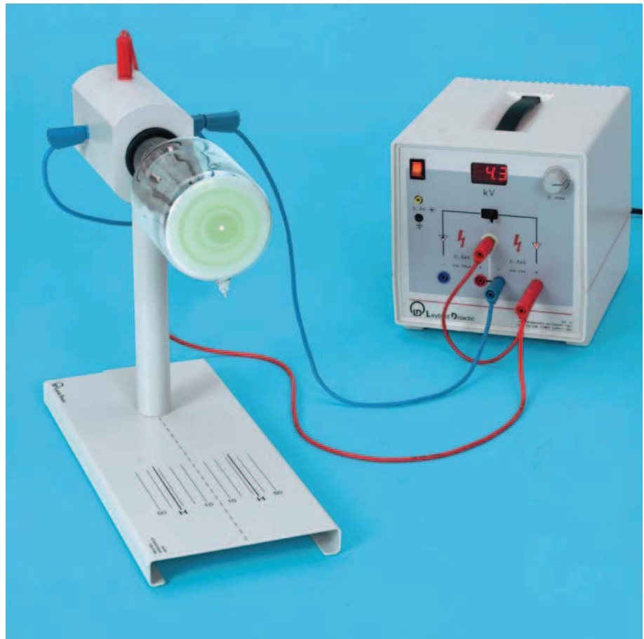
Diffraction of electrons in a polycrystalline lattice (Debye-Scherrer diffraction) (P 6.1.5.1)
