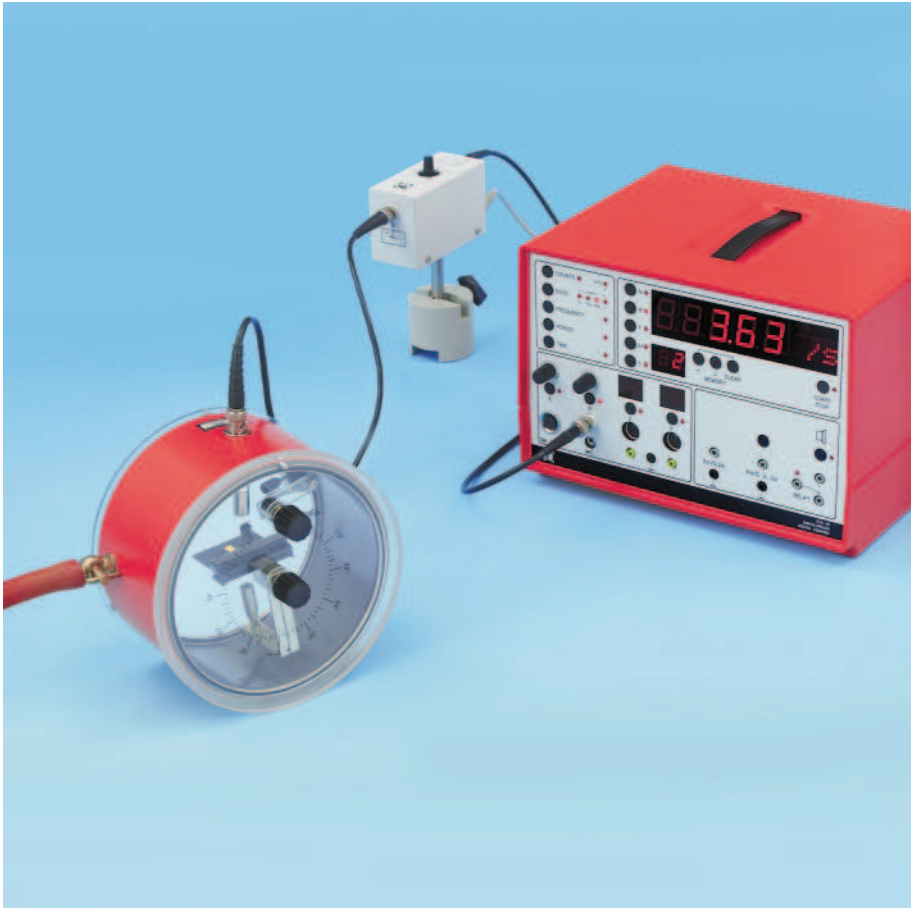
Rutherford scattering: measuring the scattering rate as a function of the scattering angle and the atomic number (P 6.5.2.1)
