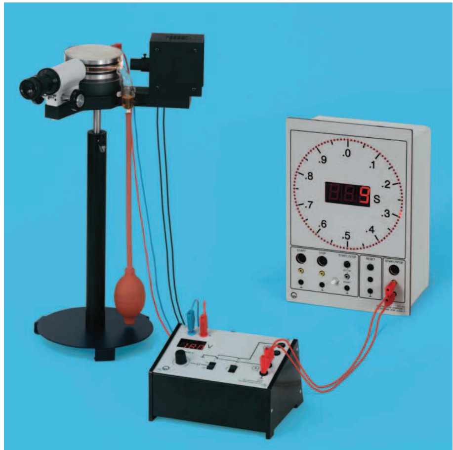
Determining the electrical charge of the electron after Millikan and demonstrating the quantum nature of the charge – measuring the suspension voltage and the falling speed (P 6.1.2.1)
