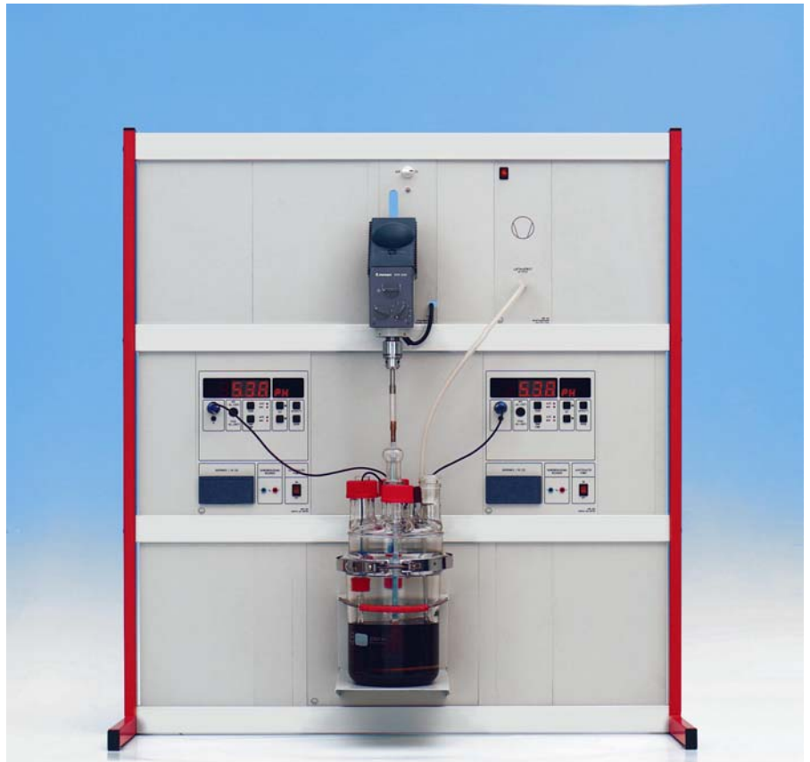
CPS experiment assembly for microbial desulfurization of coal
