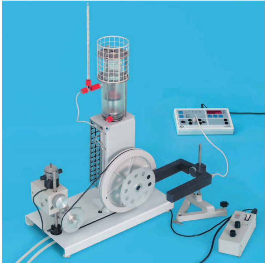
Frictional losses in the hot-air engine (calorific determination) (P 2.6.2.1)
