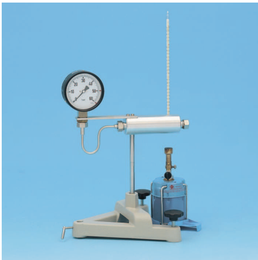
Recording the vapor pressure curve of water up to 50 bar (P 2.4.2.2)
