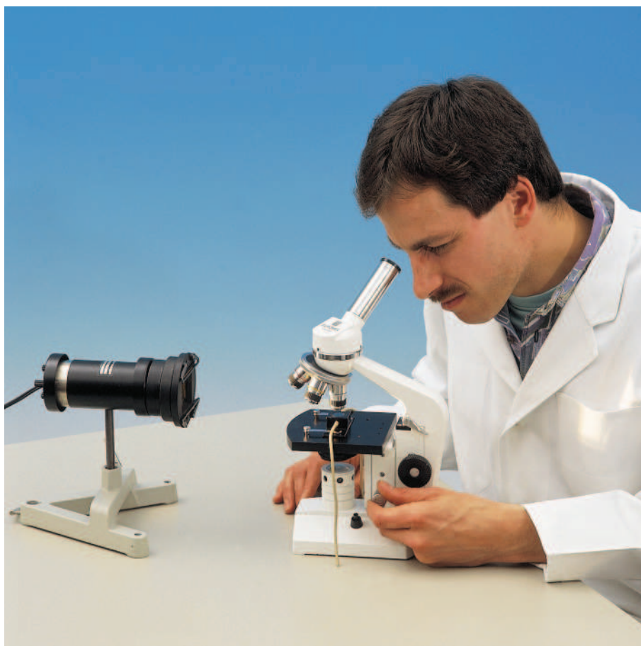
Brownian motion of smoke particles (P 2.5.1.1)
