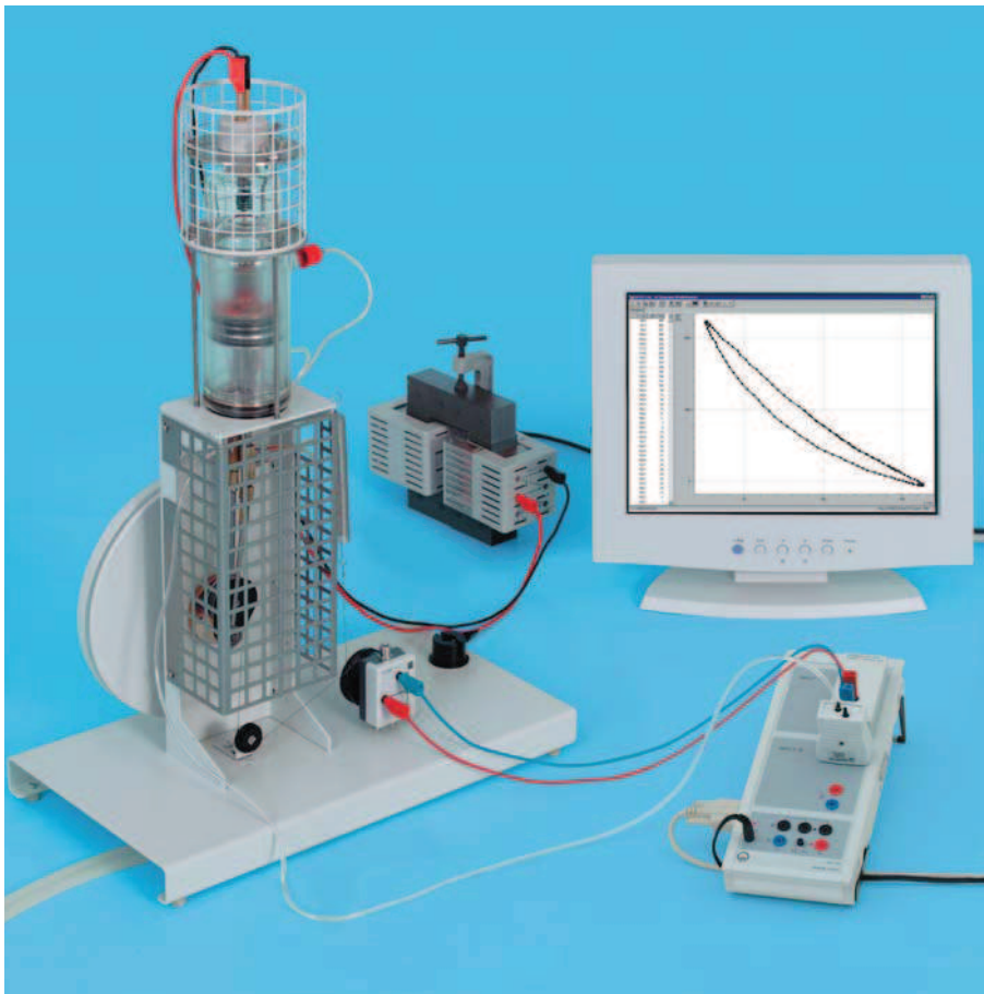
Hot-air engine as a heat engine: recording and evaluating the pV diagram with CASSY (P 2.6.2.4)
