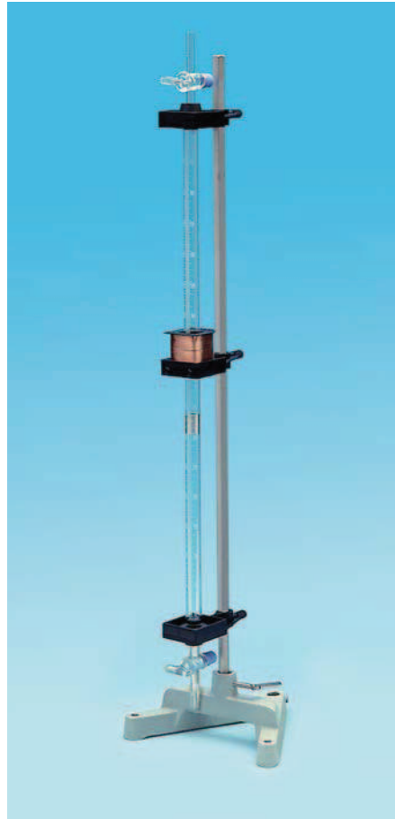
Determining the adiabatic exponent C_p/C_V of various gases using the gas elastic resonance apparatus (P 2.5.3.2)
