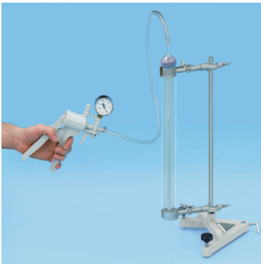
Pressure-dependency of the volume of a gas at a constant temperature (Boyle-Mariotte's law) (P 2.5.2.1)
