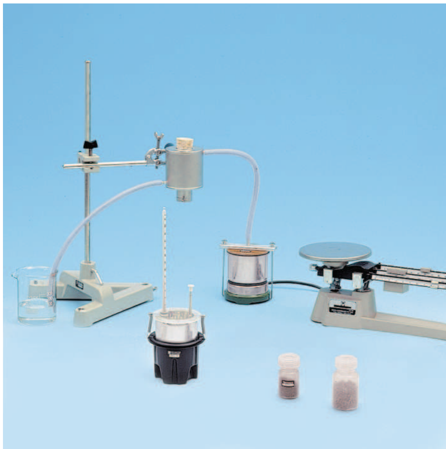
Determining the specific heat capacity of solids (P 2.3.2.1 a)
