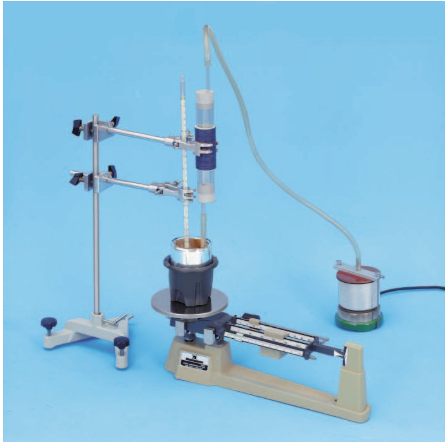
Determining the specific evaporation heat of water (P 2.4.1.1)
