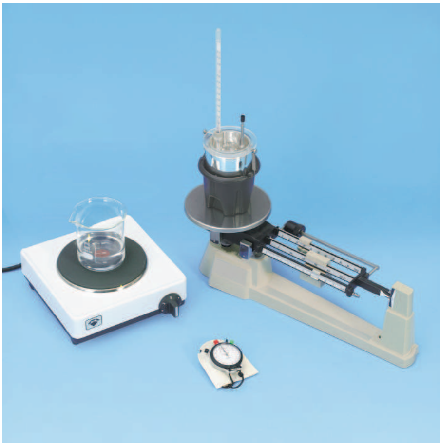
Measuring the temperature of a mixture of hot and cold water (P 2.3.1.1 a)
