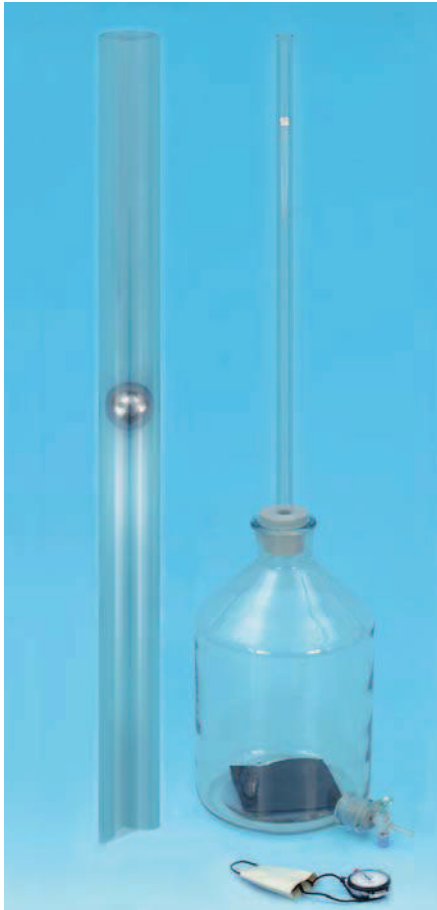
Determining the adiabatic exponent C_p/C_V of air after Rüchard (P 2.5.3.1)
