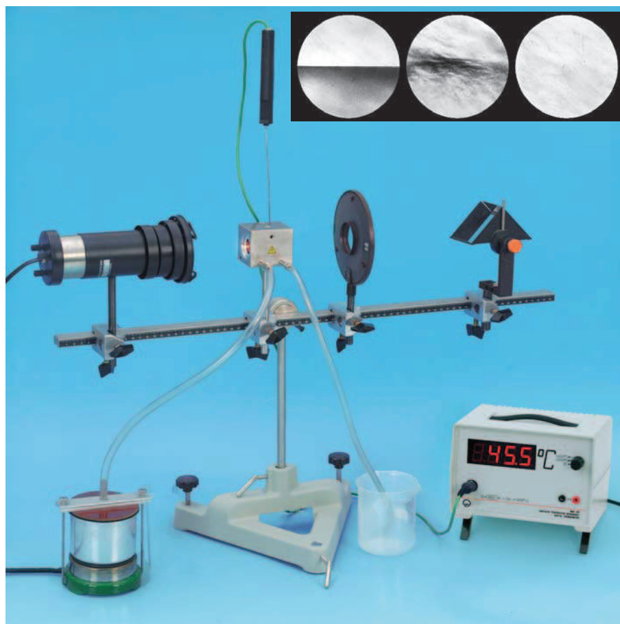
Investigating a liquid-vapor mixture at the critical point (P 2.4.3.1)
