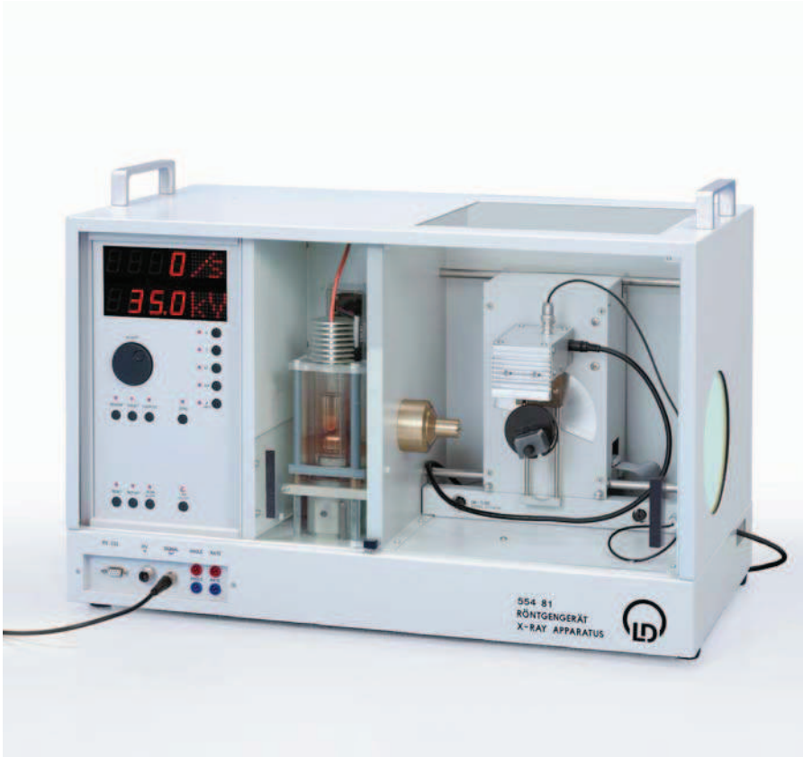
Recording of X-ray fluorescence (P 7.5.1.1+2)
