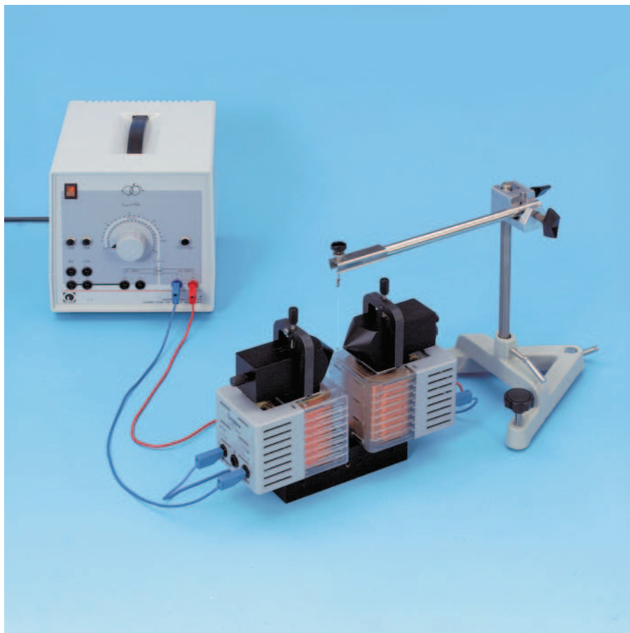
Dia-, para- and ferromagnetic materials in an inhomogeneous magnetic field (P 7.3.1.1)
