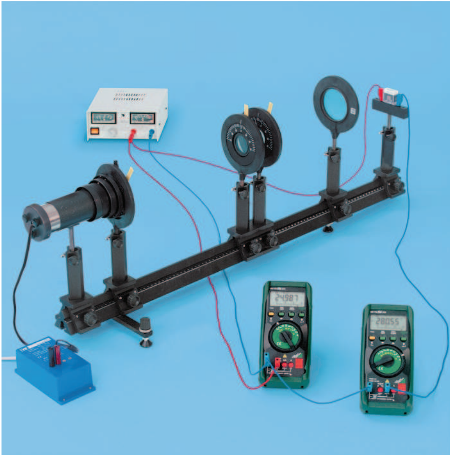
Recording the current-voltage characteristic of a CdS photoresistor (P 7.2.3.1)
