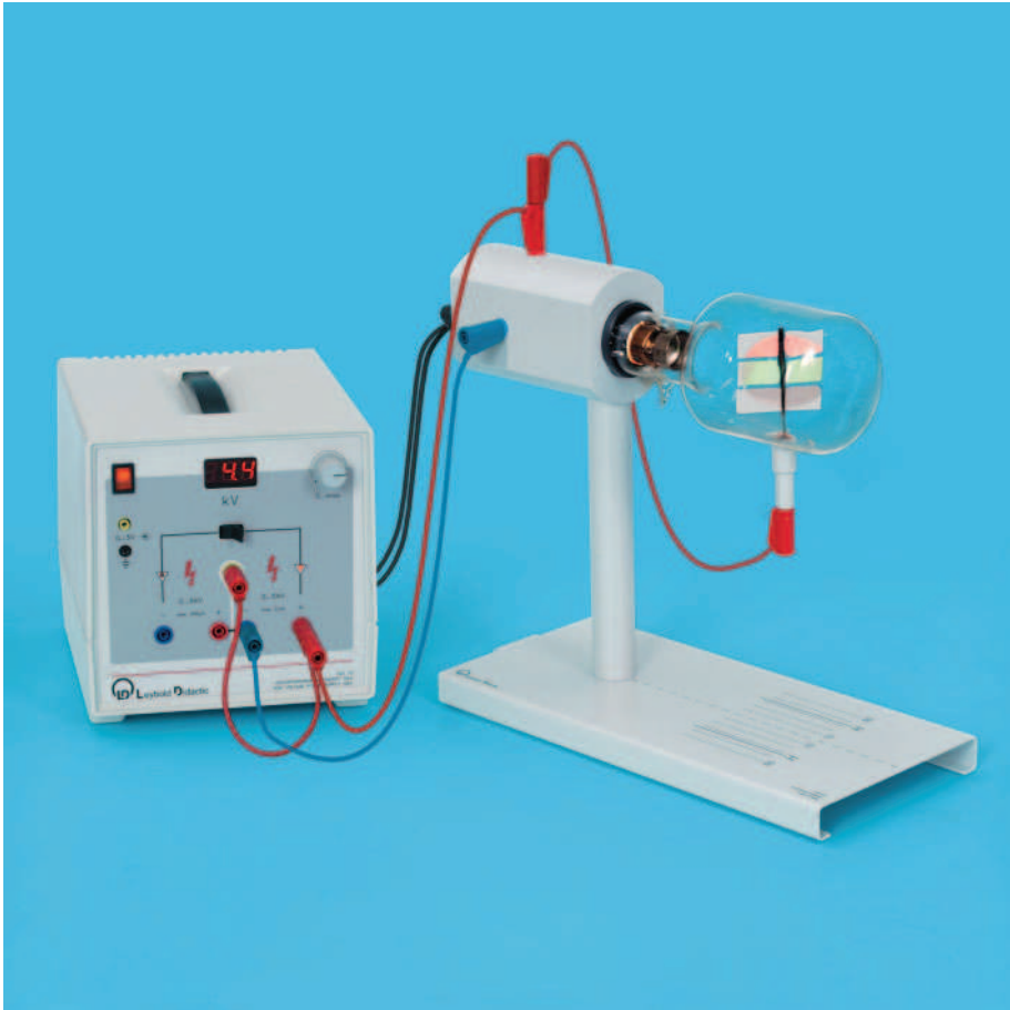
Exciting luminescence through irradiation with ultraviolet light and electrons (P 7.2.4.1)
