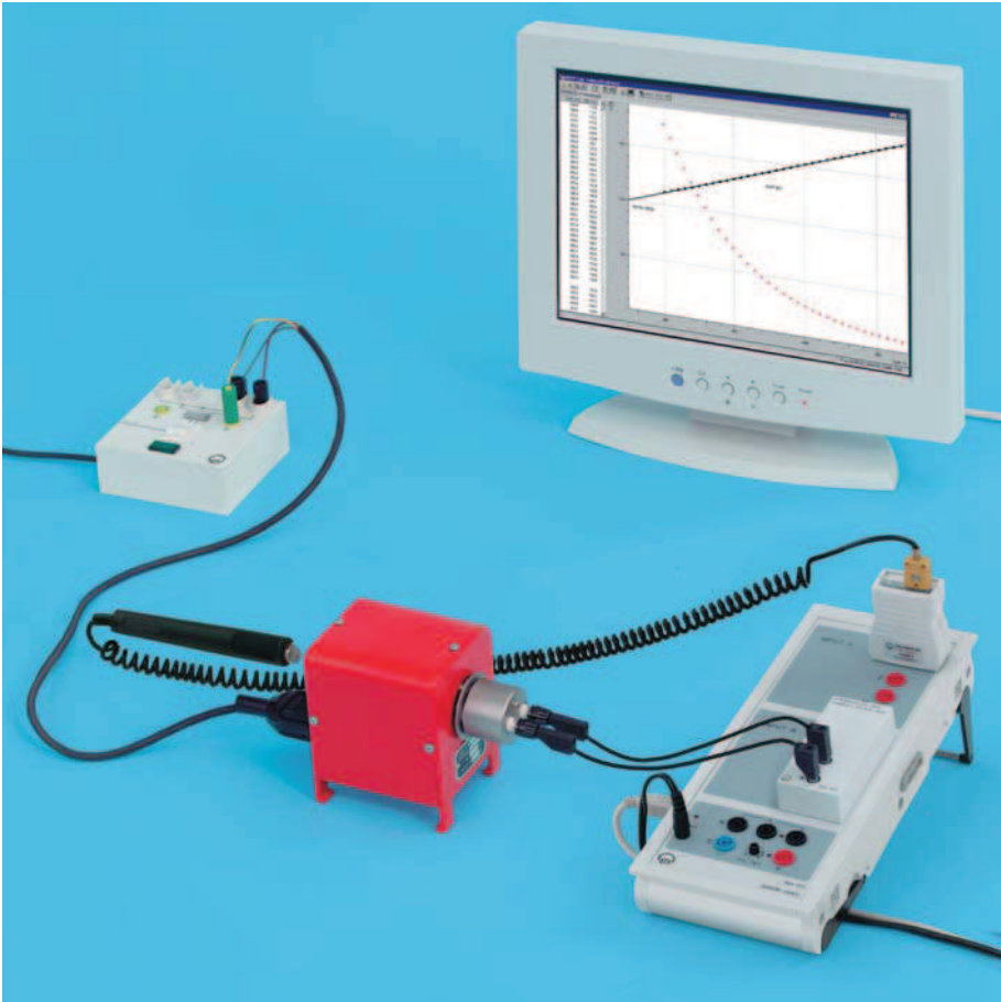
Measuring the temperature-dependency of a noble metal resistor and a semiconductor resistor (P 7.2.2.1/2)
