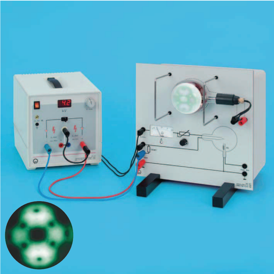
Investigating the crystal structures of tungsten using a field emission microscope (P 7.1.1.1)
