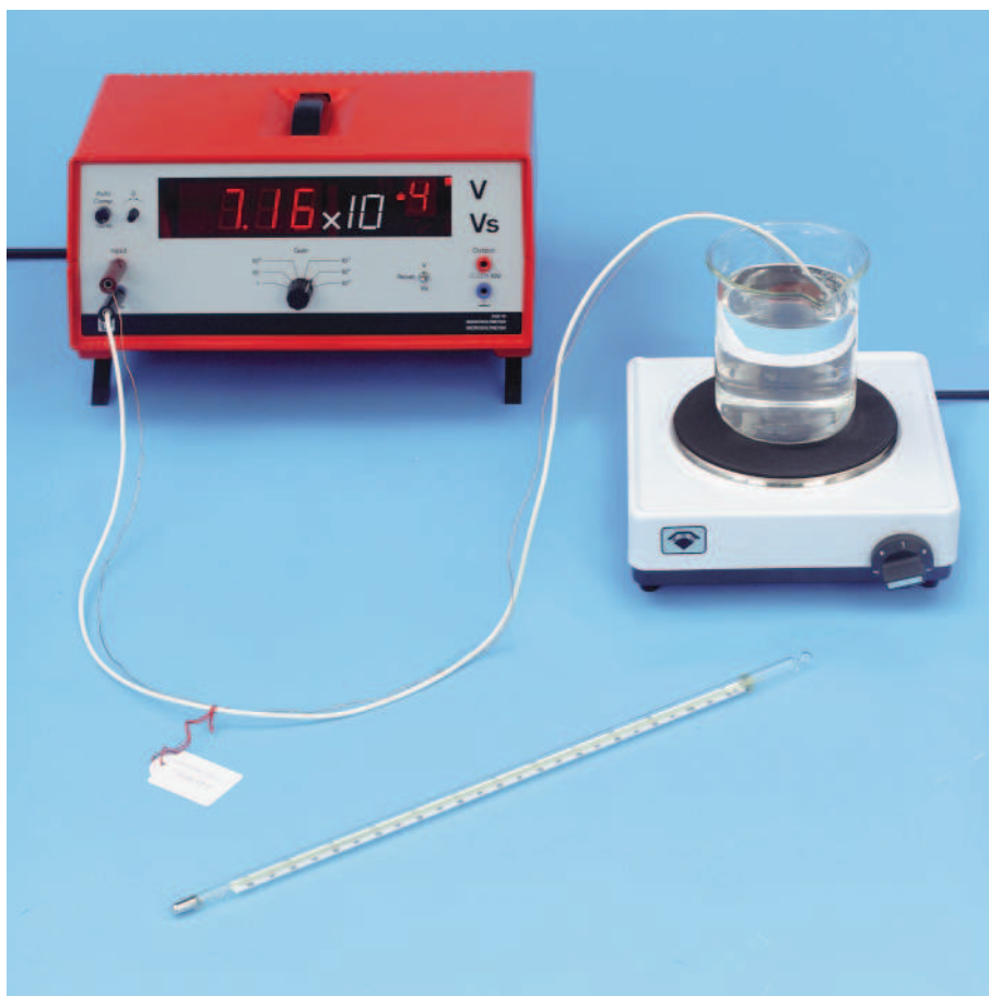
Seebeck effect: Determining the thermoelectric voltage as a function of the temperature differential (P 7.2.5.1)
